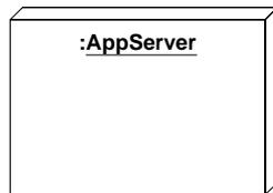
Figure 137 - An instance of a Node
