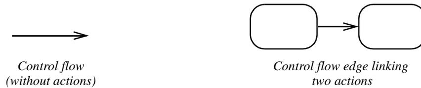
**Figure 231 - Control flow notation**
