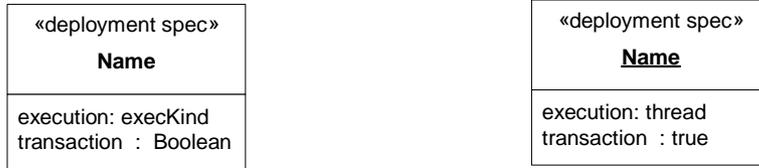
Figure 132 - A DeploymentSpecification for an artifact (specification and instance levels)
