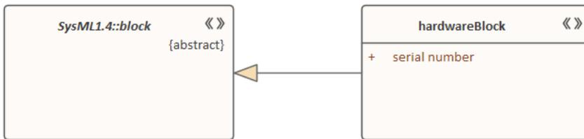
This example shows how a toolbox can allow a hardwareBlock to be created. Note that the extension is always the UML type the original stereotype extends. It is never a reference to a stereotype.
