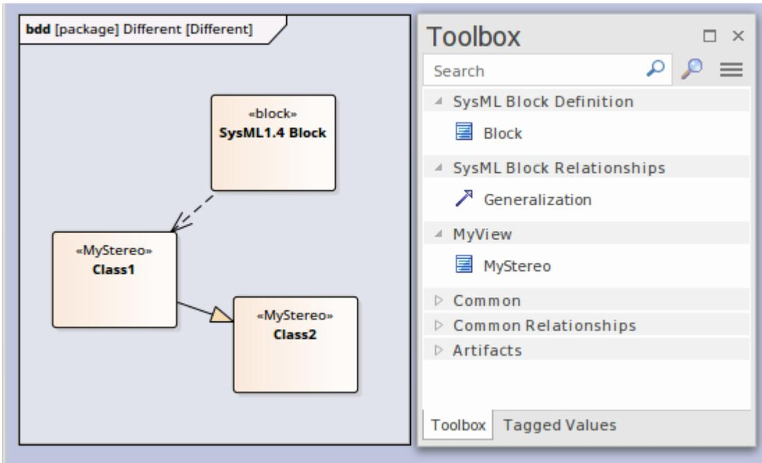
The diagram View makes the elements and connector available from the Toolbox, as shown, and from the Quick Linker. The table *Create Custom Diagram View in a Profile* explains how to create a Metamodel that defines a new diagram View, finishing with the MyView example.
