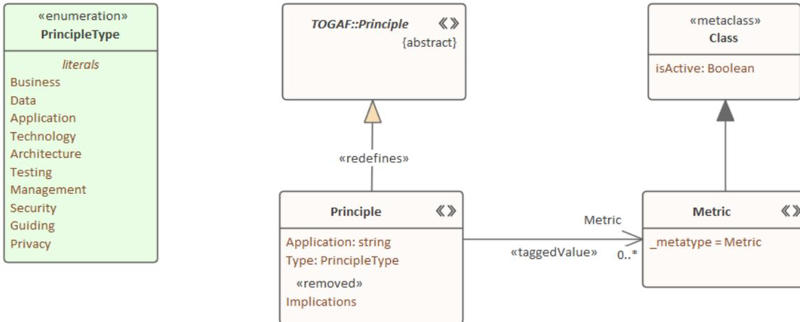
Optionally, an end user can specify that creating a TOGAF::Principle should actually create an instance of Principle from this profile. They do that by setting this profile as Active (which can only be done for a single technology.)
