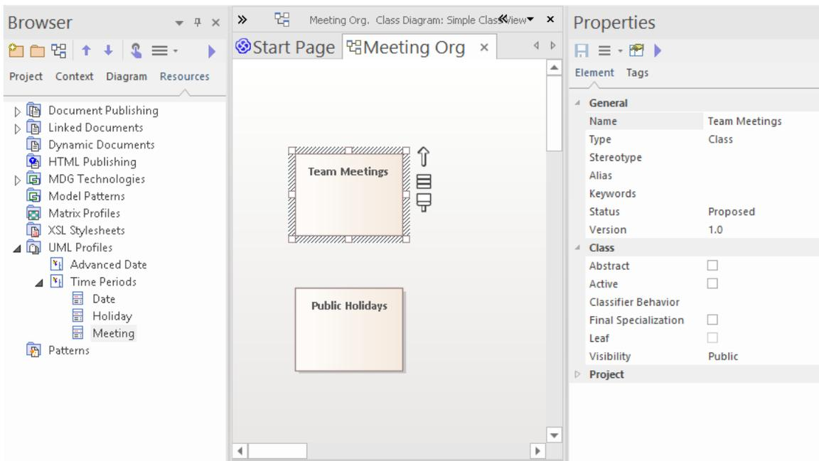
The 'Meeting' profile element is now Ctrl+dragged onto the Team Meetings Class, and the 'Holiday' profile element is Ctrl+dragged onto the Public Holidays Class. The result is that both Class elements take the appropriate stereotypes, which are displayed on the elements in the diagram and in the 'Stereotype' field on the 'Element' tab of the Properties window. Notice also that there is a stereotype group on the 'Element' tab, listing the tags defined for the stereotype.
