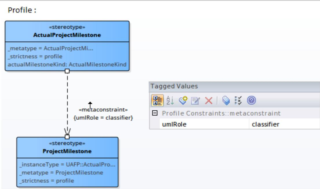
In the Profile example, a «metaconstraint» connector is drawn from ActualProjectMilestone to ProjectMilestone and the constraint is specified as classifier on the tag 'umlRole' in the connector's Tagged Values.
