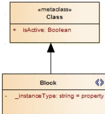
When a user drags a SysML Block element from the Browser window onto a diagram, the system checks the `_instanceType` attribute value and searches the SysML Profile for an element template with a matching `_metatype` attribute value, and generates the instance from that. With the example definition you would get a Block element with the `<<property>>` stereotype.
