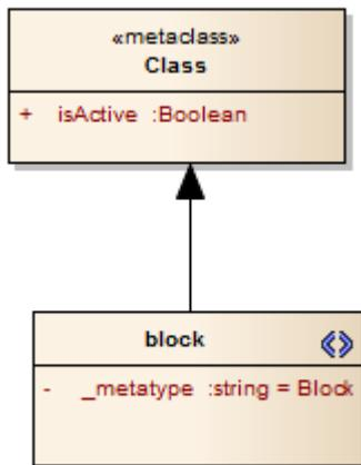
However, a SysML user is not interested in UML Classes, only in SysML Blocks. If you set the `_metatype` attribute to `Block`, any element created from that stereotype, while behaving in the same way as a stereotyped Class in most contexts, will:
