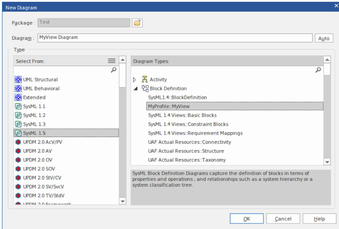
The fully extended name of the diagram View reflects the parent Profile name (MyProfile) and the View name (MyView) - hence 'MyProfile::MyView'. You could call the example View SysML 1.4 Views:: MyView to indicate that it is a member of the SysML 1.4 View suite.
