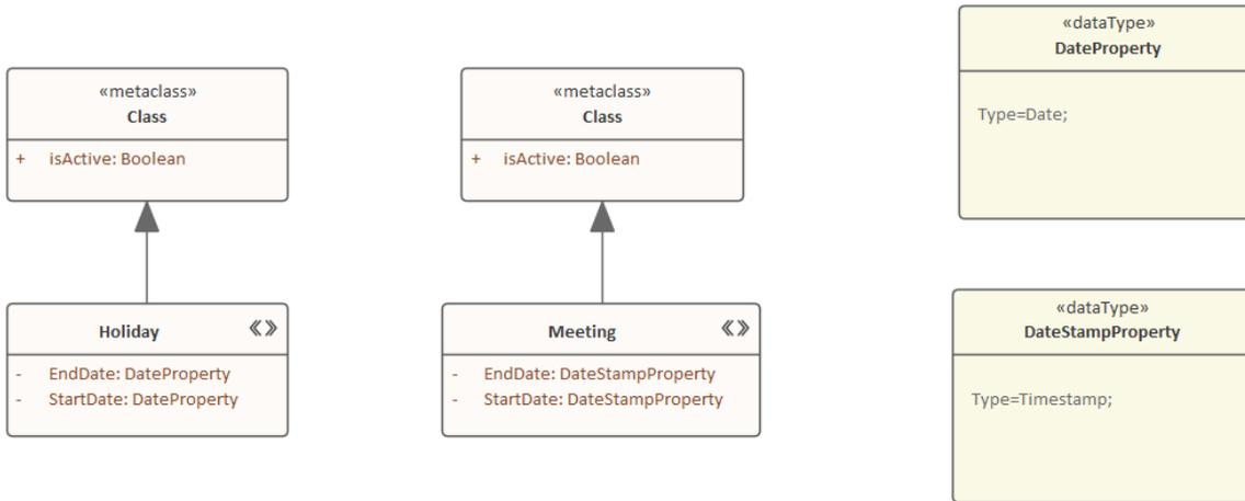
When the profile is imported into a user's model (either as a standalone profile or as a component of an MDG Technology), the stereotypes can be applied to new or existing elements, and the Tagged Value types are added (and are made available when creating more tags in the 'Tagged Value' dialog drop-down). In this illustration, the Time Periods profile has been imported into the 'Resources' tab for the model, and is about to be used to tailor two standard Class elements that exist on a diagram.
