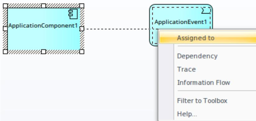
In the Profile example, a «stereotyped relationship» connector is drawn from ApplicationComponent to ApplicationEvent and the stereotype of the relationship is set to 'Assignment' in the connector's Tagged Values.
